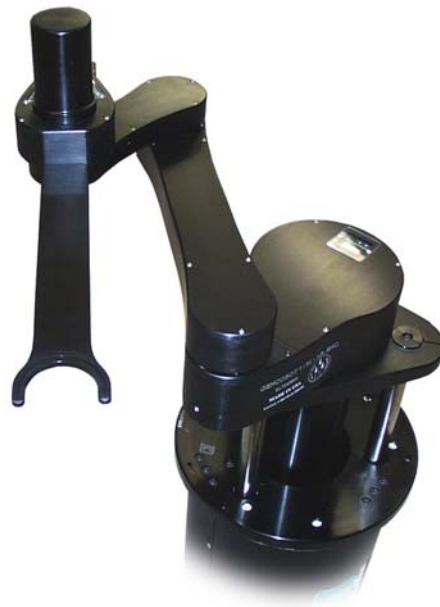
Figure1. A six-DOF GPR robot with “yaw-axis” capabilities
