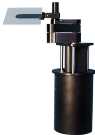
Figure 2: A 7 DOF GPR with servo controlled “roll” motion
