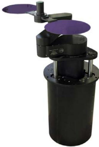
Figure 3: An extended reach, dual end-effector GPR
